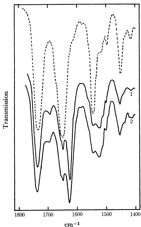
Fig. 1(a). IR spectra of PBLG-5 films cast from DMF (1) and chloroform (2) solutions. Dashed curve is that of PBLG-100 film cast from chloroform solution.
